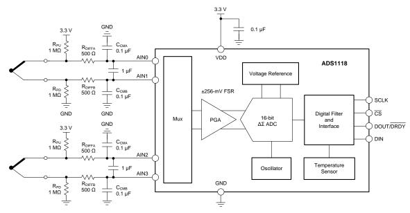
Figure 50. Two-Channel Thermocouple Measurement System
