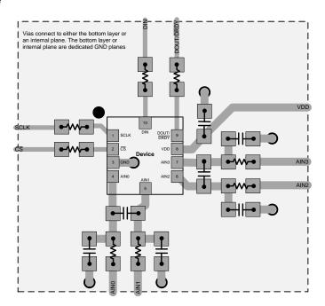
Figure 56. X2QFN Package
