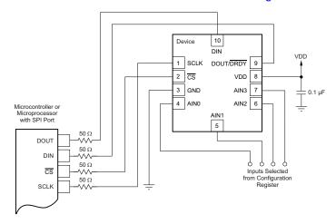
Figure 45. Typical Connections of the ADS1118
