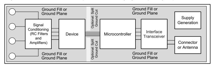
Figure 55. System Component Placement
