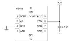
Figure 54. Power Supply Decoupling
