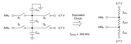
Figure 36. Simplified Analog Input Circuit
