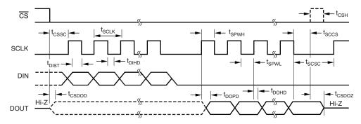
Figure 1. Serial Interface Timing
