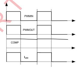
Figure 2—Fast and High Contrast Ratio PWM Dimming
