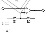
• Sample calculation Specifications - Set frequency: f = 26,000 Hz Gain at maximum boost:  $G_{+10dB} = 10$  dB Let R1 = 16.240 k $\Omega$ , R2 = 35.461 K $\Omega$ ,
