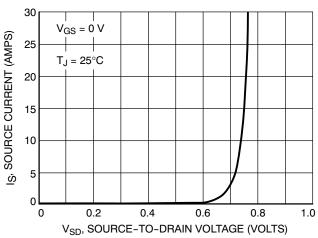
Figure 10. Diode Forward Voltage vs. Current
