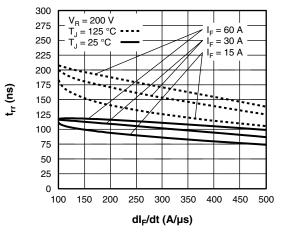
Fig. 5 - Typical Reverse Recovery Time vs. dl<sub>F</sub>/dt (Per Leg)
