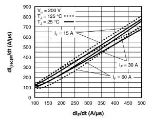
Fig. 8 - Typical  $dI_{(rec)M}/dt$  vs.  $dI_F/dt$ (Per Leg)
