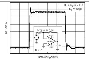
Figure 29. Small-Signal Step Response (100 mV)
