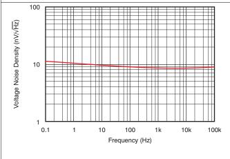
Figure 17. Input Voltage Noise Spectral Density vs Frequency
