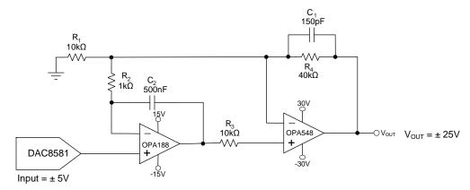
Figure 49. Programmable Power Supply
