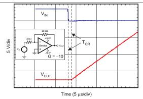
Figure 27. Positive Overload Recovery
