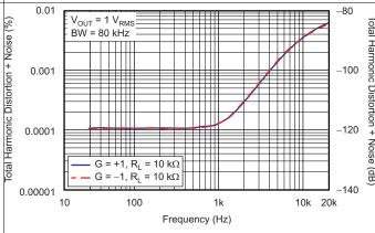
Figure 18. THD+N Ratio vs Frequency
