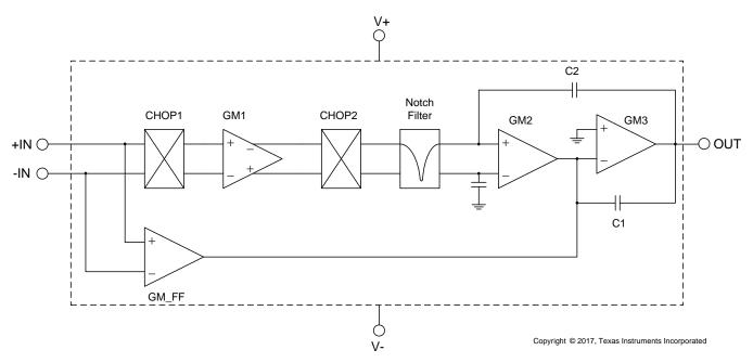
Figure 38. Functional Block Diagram
