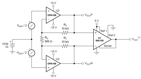
(1)  $V_{OUT} = V_{DIFF} \times (41 / 5) + (Ref 1) / 2$ .
