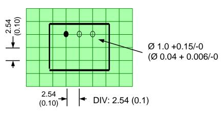
Dimensions are typical values: mm (inch) General Tolerance:  $\pm 0.25 (\pm 0.01)$ Pin Tolerance:  $\pm 0.1 (\pm 0.004)$
