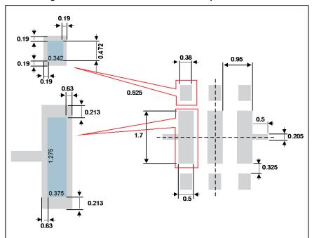
Figure 18: Recommended stencil window position in mm
