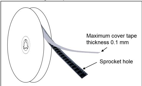
Figure 16: 13" Reel dimension definitions (mm)
