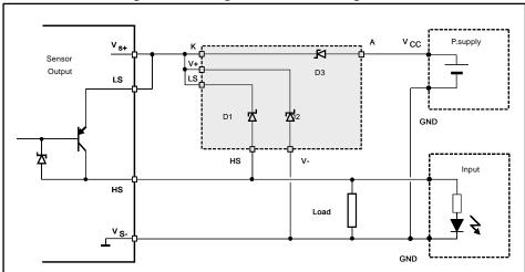
Figure 9: NPN low side sensor configuration
