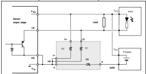
Table 6: SPT01-335 pin connection versus sensor output stage configuration as shown above
