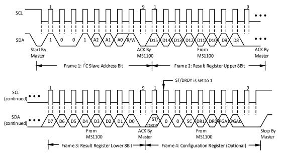
Figure 2. Timing Diagram for Reading from the MS1100
