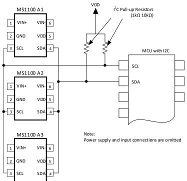
Figure 5. Connecting Multiple MS1100s
