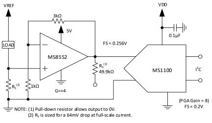
Figure 6. Low-Side Current Measurement
