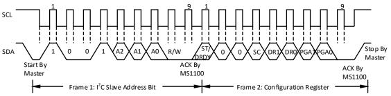
Figure 3. Timing Diagram for Writing to the MS1100
