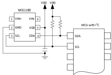
Figure 4. Typical Connections of the MS1100
