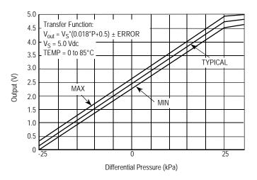
Figure 2. Output versus Pressure Differential
