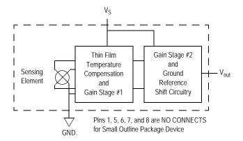
Figure 1. Fully Integrated Pressure Sensor Schematic
