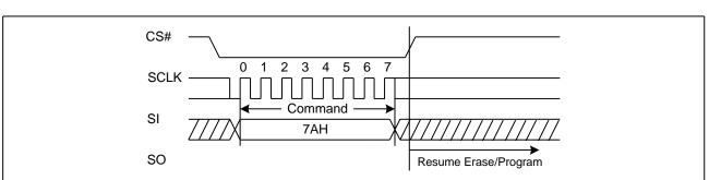
Figure 32. Program/Erase Resume Sequence Diagram
