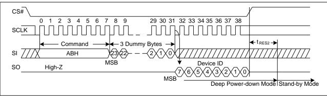
Figure 25. Release Power-Down/Read Device ID Sequence Diagram
