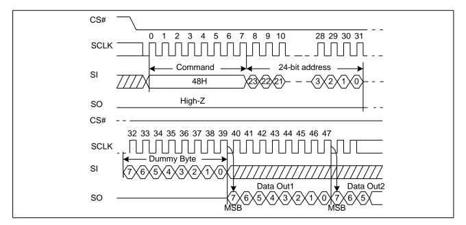
Figure35. Read Security Registers command Sequence Diagram
