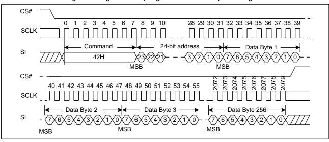
Figure34. Program Security Registers command Sequence Diagram
