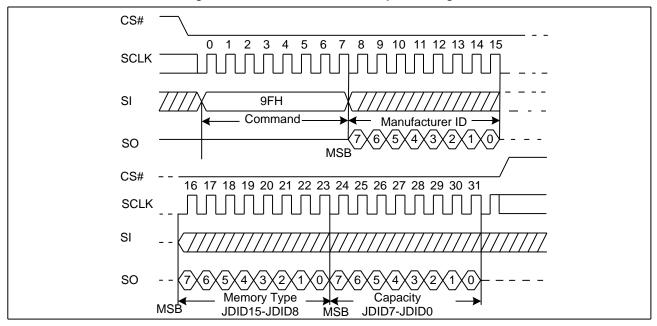
Figure27. Read Identification ID Sequence Diagram
