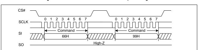
Figure36. Enable Reset and Reset command Sequence Diagram
