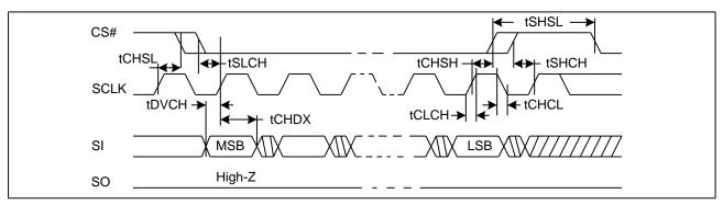
Figure41. Output Timing
