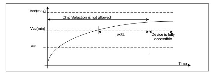
Table6. Power-Up Timing and Write Inhibit Threshold
