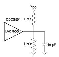
Figure 2. Test Load
