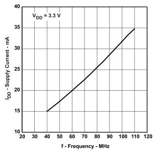
Figure 1. IDD vs. Input Frequency, VDD = 3.3V
