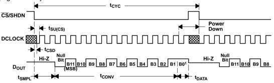
After completing the data transfer, if further clocks are applied with  $\overline{\text{CS}}$  LOW, the A/D outputs LSB-First data then followed with zeroes indefinitely.
