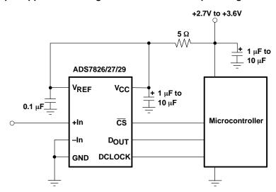
Figure 40. Basic Data Acquisition System
