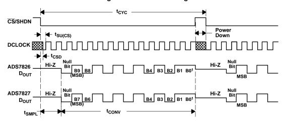
Figure 37. ADS7826 and ADS7827 Timing
