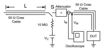
Figure 9. Simplified Schematic of a Typical TLP System
