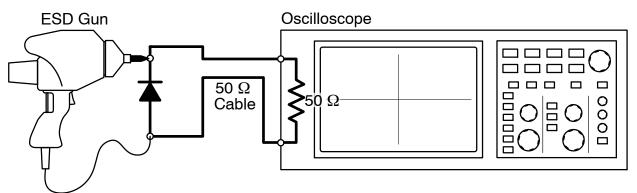
Figure 6. Diagram of ESD Clamping Voltage Test Setup
