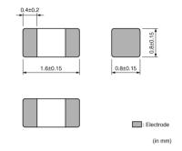
The chip ferrite beads BLM series is designed to function nearly as a resistor at noise frequencies, which greatly reduces the possibility of resonance and leaves signal wave forms undistorted.
