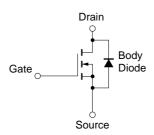
**★ Remark** Strong electric field, when exposed to this device, cause destruction of the gate oxide and ultimately degrade the device operation. Steps must be taken to stop generation of static electricity as much as possible, and quickly dissipate it once, when it has occurred.
