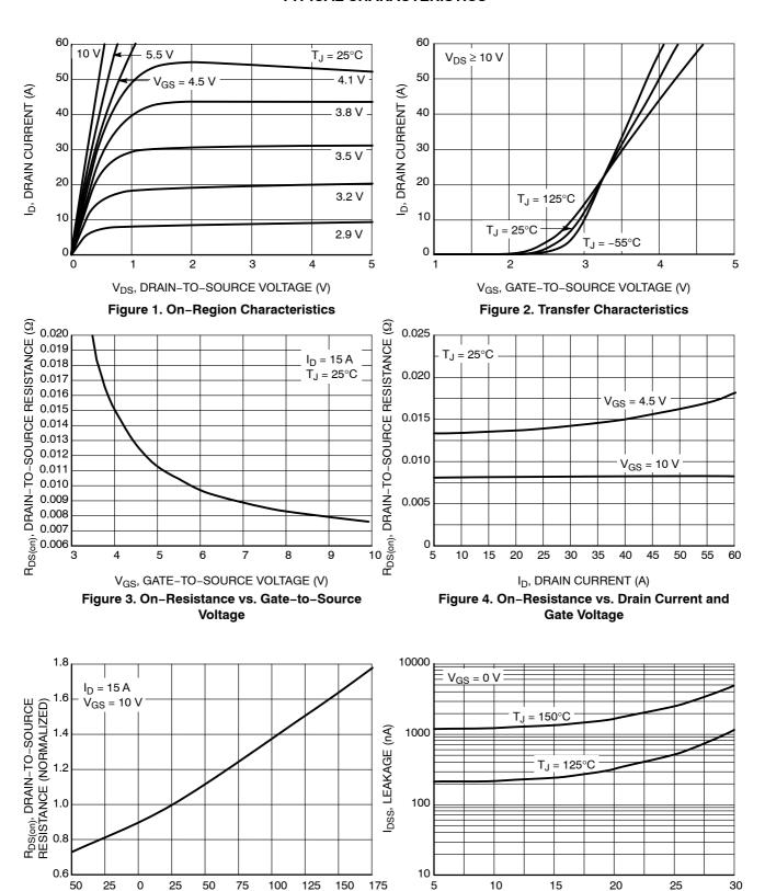
Figure 5. On–Resistance Variation with Temperature
