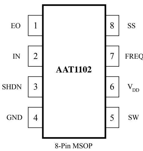
The AAT1102's versatility comes with a power-smart design. A soft-start programmed with an external capacitor that sets the input current ramp rate, reduces the current consumption to  $0.1\mu A$  in shutdown mode. When operating, a mere 2.6V input yields an impressive output voltage as high as 15V.
