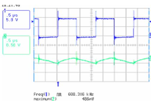
Fig.4. CH1: PWM waveform, CH2,  $v_{p-p}$
