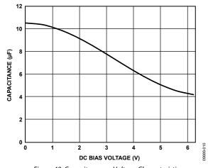
Figure 49. Capacitance vs. Voltage Characteristic
