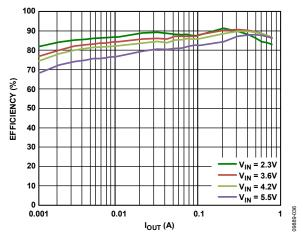
Figure 11. BUCK2 Efficiency vs. Load Current, Across Input Voltage,  $V_{\text{OUT2}} = 1.8 \text{ V}$ , Auto Mode
