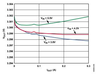
Figure 31. LDO Load Regulation Across Input Voltage,  $V_{OUT3} = 3.3 \text{ V}$
