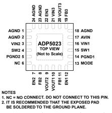
Figure 2. Pin Configuration—View from Top of Die
