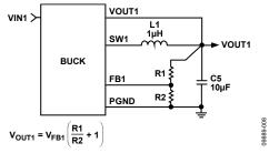
Figure 47. BUCK1 External Output Voltage Setting
