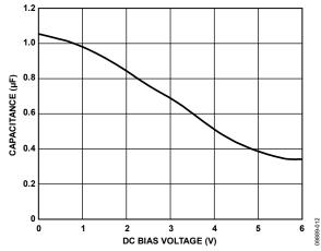
Figure 51. Capacitance vs. Voltage Characteristic
