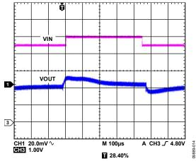
Figure 38. LDO Response to Line Transient,  $V_{IN} = 4.5 \text{ V}$  to 5 V,  $V_{OUT3} = 2.8 \text{ V}$
