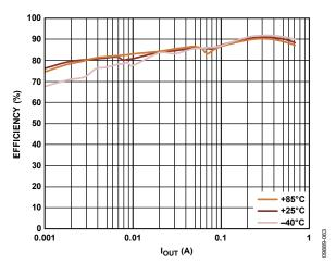
Figure 16. BUCK2 Efficiency vs. Load Current, Across Temperature,  $V_{OUZ} = 1.8 \text{ V}$ , Auto Mode
