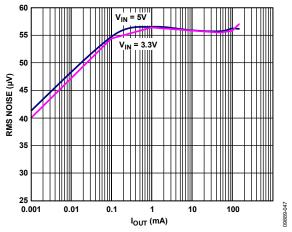
Figure 39. LDO Output Noise vs. Load Current, Across Input Voltage,  $V_{OU73} = 2.8 \text{ V}$
