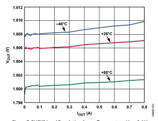
Figure 7. BUCK2 Load Regulation Across Temperature,  $V_{\text{IN}} = 3.6 \text{ V}$ ,  $V_{\text{OUT2}} = 1.8 \text{ V}$ , PWM Mode
