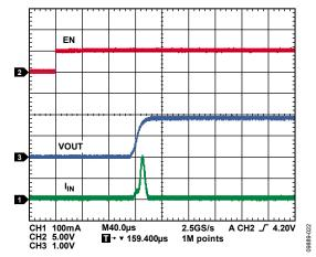
Figure 30. LDO Startup,  $V_{OUT3} = 1.8 \text{ V}$
