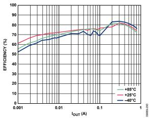
Figure 17. BUCK1 Efficiency vs. Load Current, Across Temperature, Vout1 = 0.8 V, Auto Mode
