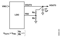
Figure 48. LDO External Output Voltage Setting
