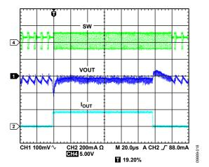
Figure 28. BUCK2 Response to Load Transient,  $I_{\rm OUT2}$  = 20 mA to 180 mA,  $V_{\rm OUT2}$  = 1.8 V, Auto Mode
