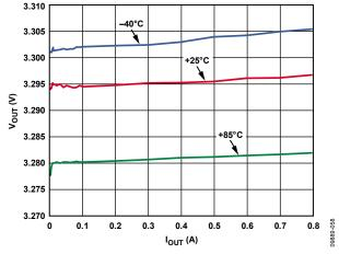
Figure 6. BUCK1 Load Regulation Across Temperature,  $V_{\text{IN}}$  = 4.2 V,  $V_{\text{OUTI}}$  = 3.3 V, PWM Mode
