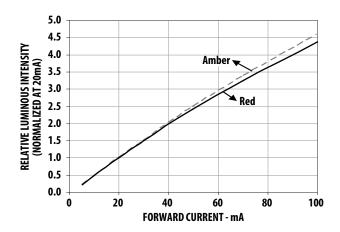
Figure 3. Relative Intensity vs Forward Current
