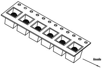
Figure 20. Unit Orientation from reel
