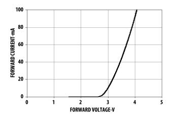
Figure 7. Forward Current vs Forward Voltage
