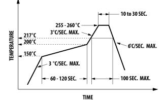
Figure 16. Recommended Leaded Reflow Soldering Profile
