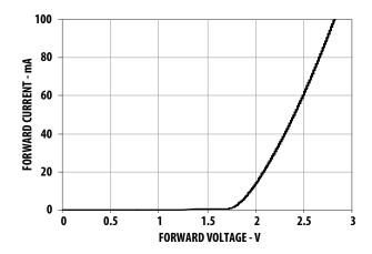
Figure 2. Forward Current vs Forward Voltage
