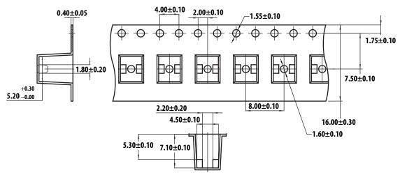
Figure 18. Carrier Tape Dimension
