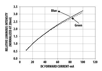
Figure 8. Relative Intensity vs Forward Current
