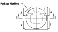
Figure 11b. Component Axis for Radiation Pattern
