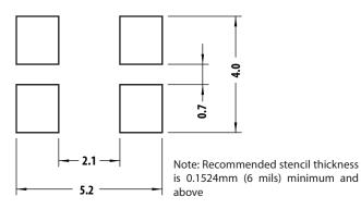
Figure 14. Recommended Soldering Land Pattern
