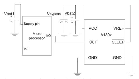
Figure 2. Application circuit showing sleep mode disabled and output ratiometirc to the A139x supply.
