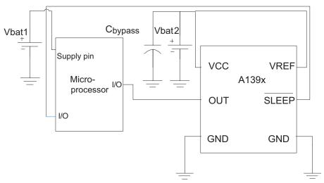
Figure 3. Application circuit showing microprocessor-controlled sleep mode and output ratiometirc to the A139x supply.
