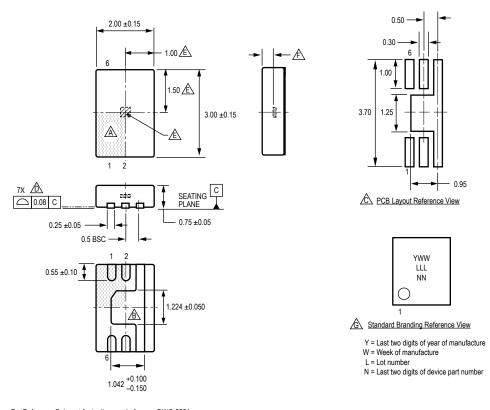
For Reference Only, not for tooling use (reference DWG-2861; reference JEDEC MO-229WCED, Type 1) Dimensions in millimeters
