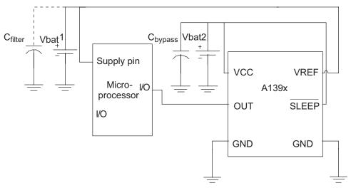
Figure 4. Application circuit showing ratiometry of  $V_{REF}$ . Sleep mode is disabled and the VREF pin is tied to the microprocessor supply.
