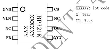
Figure 2. Pin configuration
