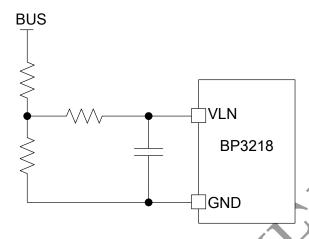
Figure 4. VLN pin application circuit
