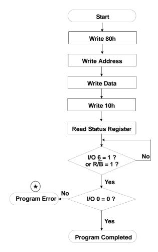
: If program operation results in an error, map out the block including the page in error and copy the target data to another block.
