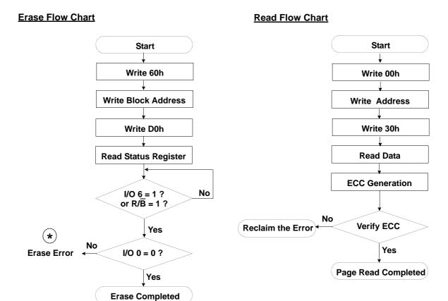
\* : If erase operation results in an error, map out the failing block and replace it with another block.
