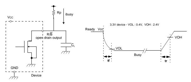
[Figure 12] Rp vs tr ,tf & Rp vs ibusy
