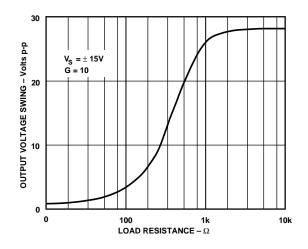
Figure 18. Output Voltage Swing vs. Resistive Load
