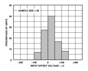
Figure 1. Typical Distribution of  $V_{OS}$ , Gain = 10
