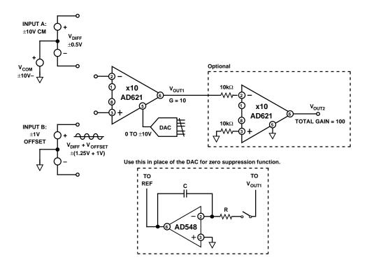
Figure 32. Suppressing a Large Common-Mode or Offset Voltage in Order to Measure a Small Differential Signal ( $V_S = \pm 15 \text{ V}$ )
