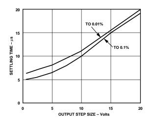
Figure 23. Settling Time vs. Step Size, G = 10
