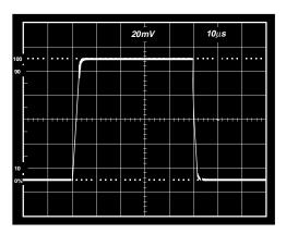
Figure 22. Small Signal Pulse Response, G = 100,  $R_L$  = 2 k $\Omega$ ,  $C_L$  = 100 pF
