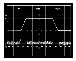
Figure 19. Large Signal Pulse Response and Settling Time Gain, G = 10 (0.5 mV = 0.01%),  $R_L$  = 1 k  $\Omega$ ,  $C_L$  = 100 pF
