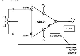
Figure 42a. Ground Returns for Bias Currents when Using Transformer Input Coupling
