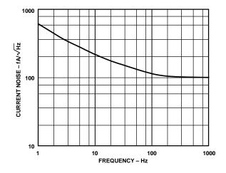
Figure 7. Current Noise Spectral Density vs. Frequency
