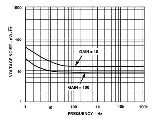
Figure 6. Voltage Noise Spectral Density
