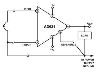
Figure 42b. Ground Returns for Bias Currents when Using a Thermocouple Input
