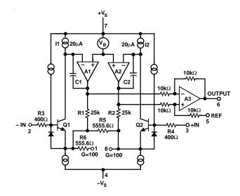
Figure 29. Simplified Schematic of AD621
