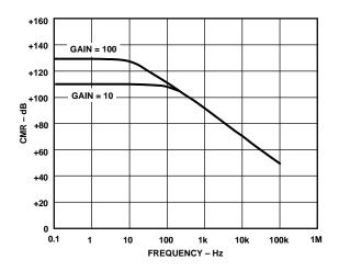
Figure 11. CMR vs. Frequency, RTI, for a Zero to 1  $k\!\Omega$  Source Imbalance
