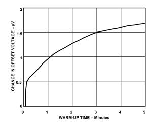
Figure 5. Change in Input Offset Voltage vs. Warm-Up Time
