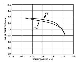
Figure 25. Input Bias Current vs. Temperature
