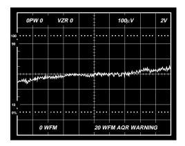
Figure 26. Gain Nonlinearity, G = 100,  $R_L = 10 \ k\Omega$ ,  $C_L = 0 \ pF$ . Vertical Scale:  $100 \ \mu V/Div = 100 \ ppm/Div$ Horizontal Scale:  $2 \ Volts/Div$
