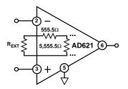
Figure 37. Programming the AD621 for Gains Between 10 and 100
