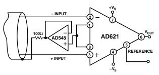
Figure 40. Common-Mode Shield Driver, G = 100
