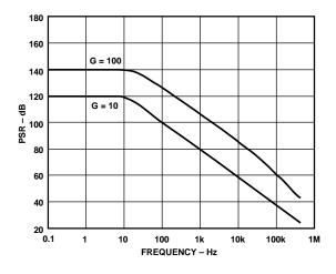
Figure 13. Negative PSR vs. Frequency
