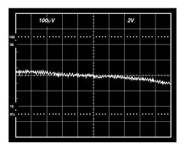
Figure 27. Gain Nonlinearity, G = 10,  $R_L$  = 10 k $\Omega$ , Vertical Scale: 100  $\mu$ V/Div = 100 ppm/Div, Horizontal Scale: 2 Volts/Div
