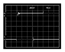
Figure 20. Small Signal Pulse Response, G = 10,  $R_L = 1 k \Omega$ ,  $C_L = 100 pF$
