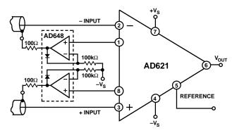
Figure 39. Differential Shield Driver, G = 10
