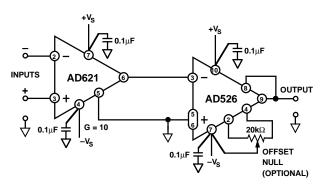
Figure 38. A High Performance Programmable Gain Amplifier
