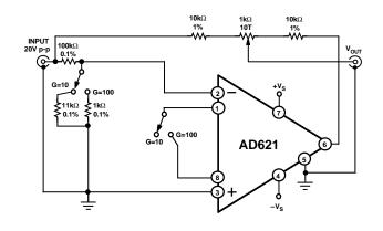
Figure 28. Settling Time Test Circuit
