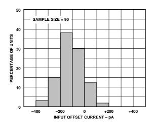
Figure 3. Typical Distribution of Input Offset Current
