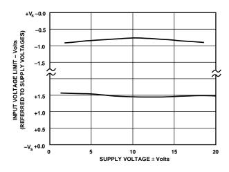
Figure 16. Input Voltage Range vs. Supply Voltage
