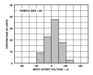
Figure 2. Typical Distribution of  $V_{OS}$ , Gain = 100
