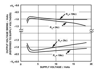
Figure 17. Output Voltage Swing vs. Supply Voltage, G = 10
