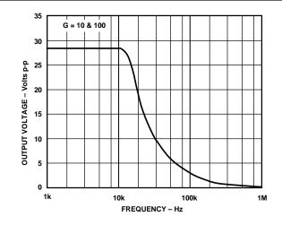
Figure 15. Large Signal Frequency Response
