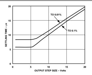
Figure 24. Settling Time vs. Step Size, Gain = 100
