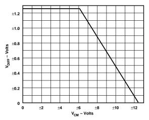
Figure 34. Trade-Off Between  $V_{CM}$  and  $V_{DIFF}$  Range ( $V_S = \pm 15 V$ , G = 10), for Reference Pin at Ground
