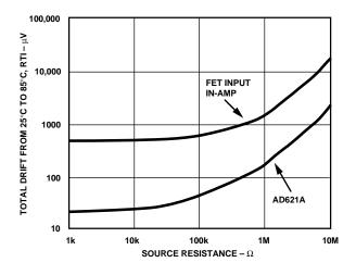
Figure 10. Total Drift vs. Source Resistance
