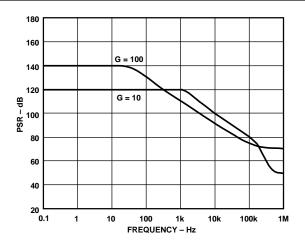
Figure 12. Positive PSR vs. Frequency
