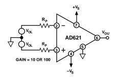
Figure 36. Input Overload Protection
