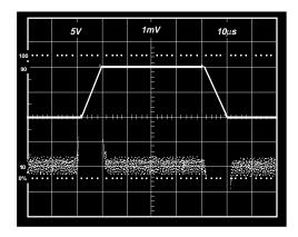
Figure 21. Large Signal Pulse Response and Settling Time, G = 100 (0.5 mV = 0.1%),  $R_L = 2 \text{ k}\Omega$ ,  $C_L = 100 \text{ pF}$
