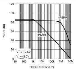
Figure 21. PSRR vs. Frequency
