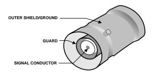
Figure 49. The Structure of a Triax
