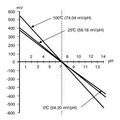
Figure 51. pH Electrode Transfer Function
