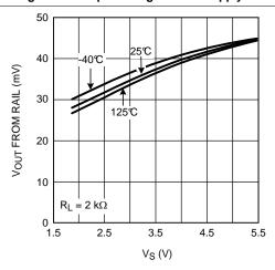
Figure 41. Output Swing Low vs. Supply Voltage
