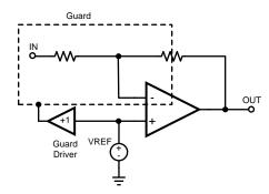
Figure 48. Guarding the Inverting or Transimpedance Configuration
