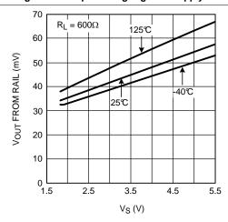
Figure 42. Output Swing High vs. Supply Voltage
