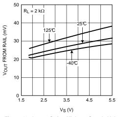
Figure 40. Output Swing High vs. Supply Voltage
