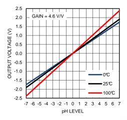
Figure 53. Output Voltage vs. pH Level
