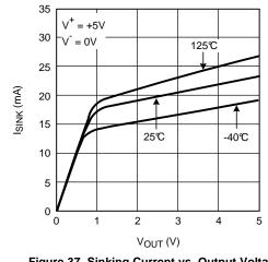
Figure 37. Sinking Current vs. Output Voltage
