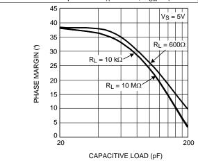
Figure 19. Phase Margin vs. Capacitive Load
