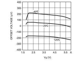
Figure 13. Offset Voltage vs. Supply Voltage
