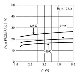
Figure 38. Output Swing High vs. Supply Voltage
