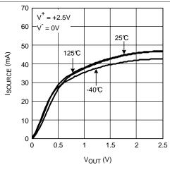
Figure 34. Sourcing Current vs. Output Voltage
