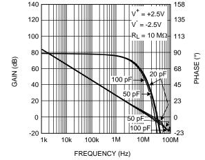
Figure 16. Open-Loop Frequency Response Gain and Phase
