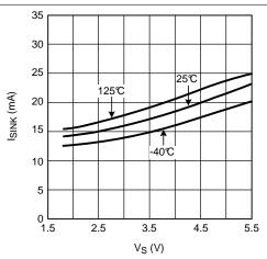
Figure 33. Sinking Current vs. Supply Voltage
