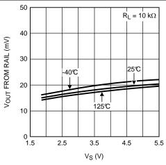
Figure 39. Output Swing Low vs. Supply Voltage
