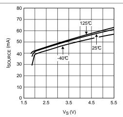
Figure 32. Sourcing Current vs. Supply Voltage
