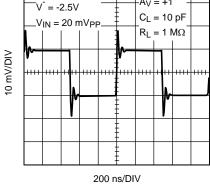
Figure 24. Small Signal Step Response
