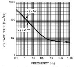
Figure 22. Input-Referred Voltage Noise vs. Frequency
