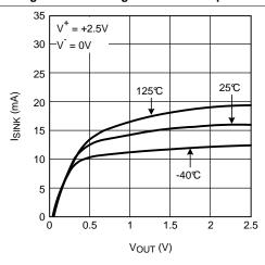
Figure 36. Sinking Current vs. Output Voltage
