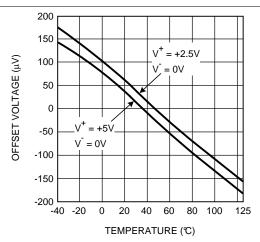
Figure 14. Offset Voltage vs. Temperature
