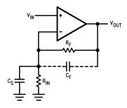
Figure 45. General Operational Amplifier Circuit
