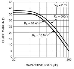
Figure 18. Phase Margin vs. Capacitive Load
