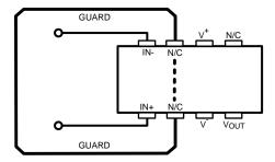
Figure 54. Layout Example Showing Guard Trace
