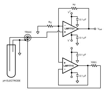
Figure 50. LMP7721 as pH Electrode Amplifier
