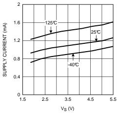
Figure 15. Supply Current vs. Supply Voltage
