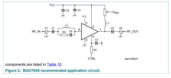
(Values can be changed depending on the PCB routing) Keep the components (L2, R3, C6) next to the BGU7045 RF input pin.
