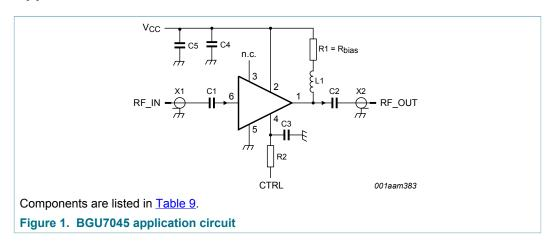
All control and supply lines must be decoupled properly. The decoupling capacitors must be placed as close to the device as possible.
