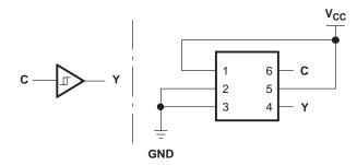
Figure 8. Noninverted Buffer
