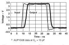
Switching Characteristics at 25 MHz<sup>†</sup>
