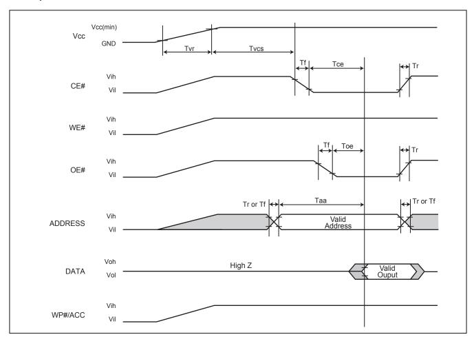
Figure A. AC Timing at Device Power-Up
