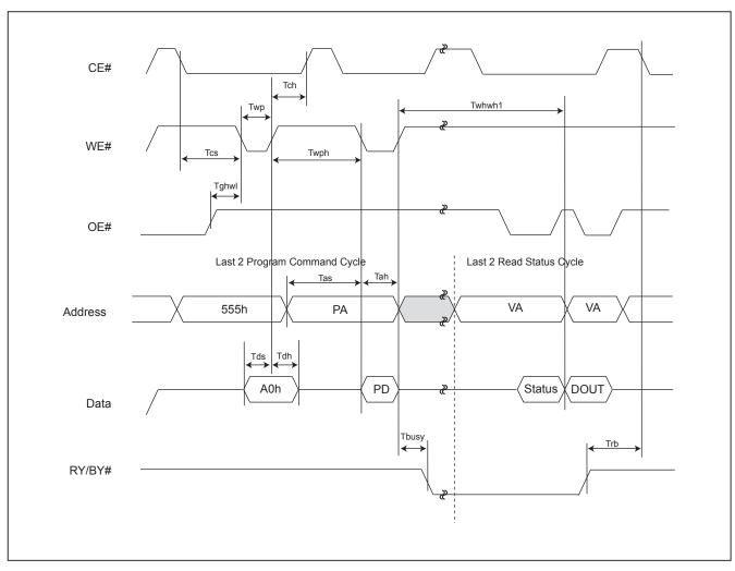
Figure 10. ACCELERATED PROGRAM TIMING DIAGRAM
