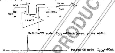
When the potential on pin 3 is decreased abruptly by turning the power switch OFF as shown above, potential reversal between pin 0 and pin 3 will occur, causing reverse current  $I_{CCX}$  to flow into the IC system. This loads the IC heavily,
