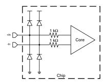
Figure 2. Equivalent Input Structure
