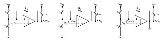
Figure 5. Inverting Configuration with Hysteresis
