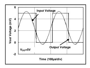
Figure 1. Comparator Response to Input Voltage
