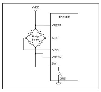
Figure 15. Low-Side Power Switch
