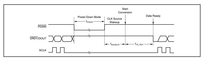
Figure 23. Wake-Up Timing from Power-Down Mode
