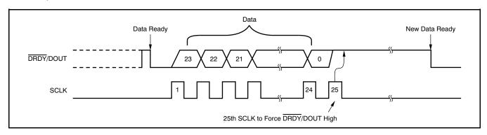
Figure 20. Data Retrieval with DRDY/DOUT Forced High Afterwards
