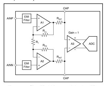
Figure 13. Simplified Diagram of the Amplifier
