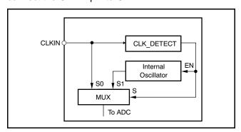
Figure 16. Equivalent Circuitry of the Clock Source
