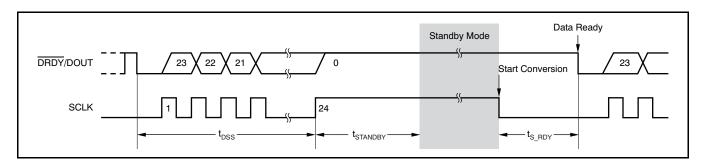
Figure 21. Standby Mode Timing (Can be used for single conversions)
