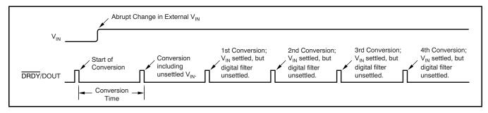
Figure 18. Settling Time in Continuous Conversion Mode
