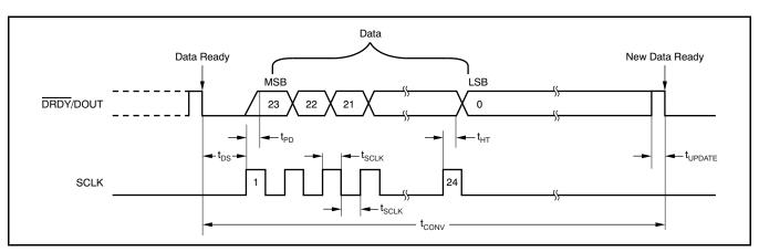
Figure 19. 24-Bit Data Retrieval Timing
