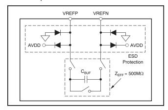
Figure 14. Simplified Reference Input Circuitry
