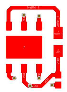
Figure 11-2. HDC2080 PCB Layout Example
