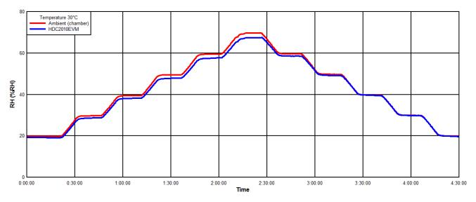
Figure 9-2. RH% Readings of Chamber and HDC2080 vs. Time
