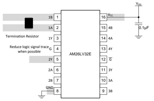
Figure 6. Trace Layout on PCB and Recommendations
