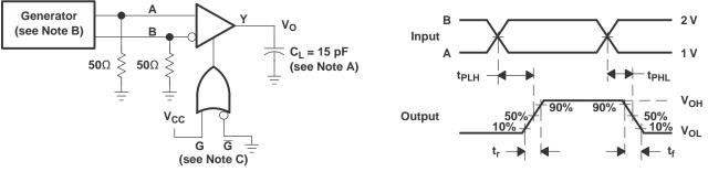
A. C<sub>L</sub> includes probe and jig capacitance.
