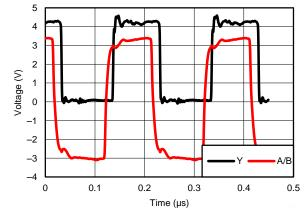
Figure 5. Differential 120- $\Omega$  Terminated Output Waveforms (CAT 5E Cable)
