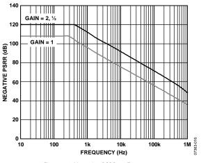
Figure 20. Negative PSRR vs. Frequency
