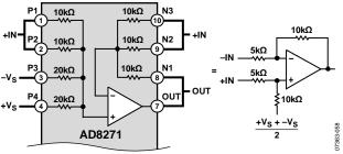
*Figure 50. Gain = 2 Difference Amplifier, Referenced to Midsupply*
