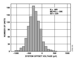
*Figure 5. Typical Distribution of System Offset, Gain = 1*
