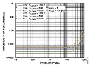
Figure 39. Harmonic Distortion Products vs. Frequency, Gain = 1
