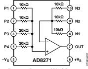
Figure 43. Functional Block Diagram
