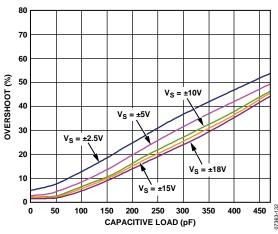
Figure 30. Small-Signal Overshoot vs. Capacitive Load, Gain = 2
