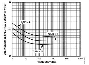
Figure 35. Voltage Noise Spectral Density vs. Frequency, Referred to Output
