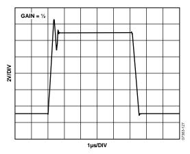
Figure 31. Large-Signal Pulse Response, Gain = 1/2
