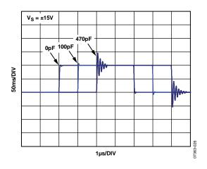
Figure 27. Small-Signal Step Response, Gain = 2
