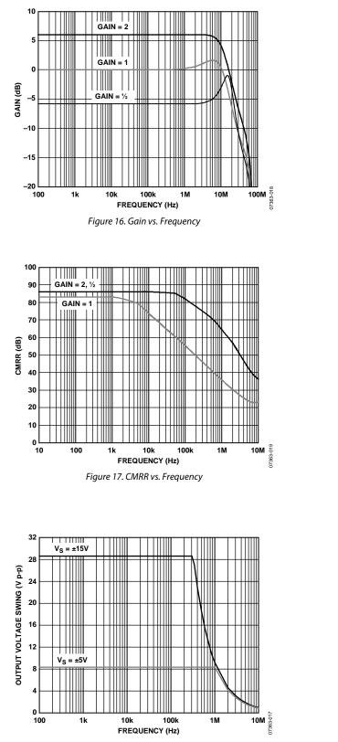
Figure 18. Output Voltage Swing vs. Large-Signal Frequency Response
