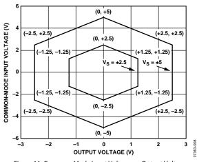
Figure 11. Common-Mode Input Voltage vs. Output Voltage, Gain =  $\frac{1}{2}$ ,  $\pm 5$  V and  $\pm 2.5$  V Supplies
