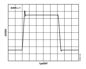
Figure 32. Large-Signal Pulse Response, Gain = 1
