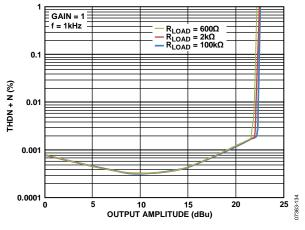
Figure 38. THD + N vs. Output Amplitude, Gain = 1
