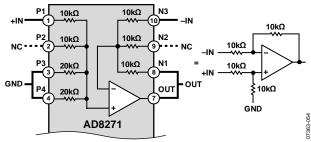
Figure 46. Gain = 1 Difference Amplifier, Referenced to Ground
