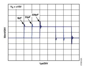
Figure 26. Small-Signal Step Response, Gain = 1
