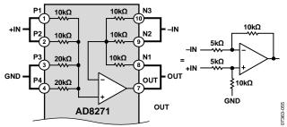
Figure 47. Gain = 2 Difference Amplifier, Referenced to Ground
