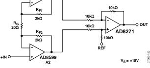
Figure 53.Ultralow Noise Instrumentation Amplifier Using AD8599 Configured for Gain = 201
