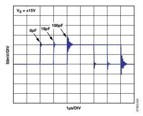
Figure 25. Small-Signal Step Response, Gain =  $\frac{1}{2}$
