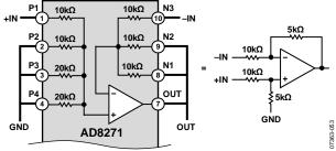
Figure 45. Gain = 1/2 Difference Amplifier, Referenced to Ground
