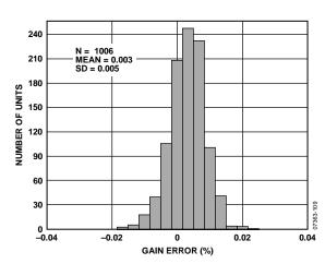
Figure 6. Typical Distribution of Gain Error, Gain = 1
