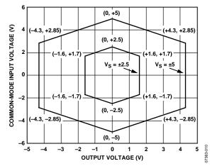
Figure 13. Common-Mode Input Voltage vs. Output Voltage, Gain = 1, ±5 V and ±2.5 V Supplies
