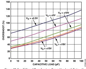
Figure 28. Small-Signal Overshoot vs. Capacitive Load, Gain =  $\frac{1}{2}$
