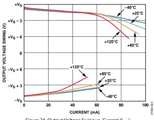
Figure 24. Output Voltage Swing vs. Current (IOUT)
