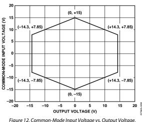
Figure 12. Common-Mode Input Voltage vs. Output Voltage, Gain = 1,  $\pm$ 15 V Supplies
