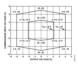
Figure 15. Common-Mode Input Voltage vs. Output Voltage, Gain = 2,  $\pm$ 5 V and  $\pm$ 2.5 V Supplies
