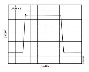
Figure 33. Large-Signal Pulse Response, Gain = 2
