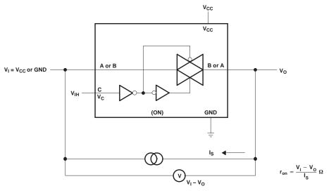
Figure 2. ON-State Resistance Test Circuit
