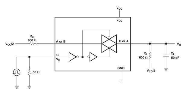
Figure 7. Crosstalk (Control Input – Switch Output)
