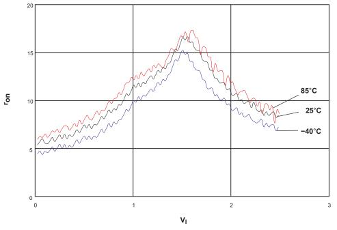
Figure 12.  $r_{on}$  vs V<sub>I</sub>, V<sub>CC</sub> = 2.5 V (SN74LVC1G66-Q1)
