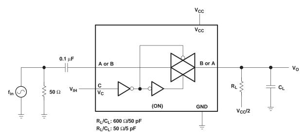
Figure 6. Frequency Response (Switch ON)
