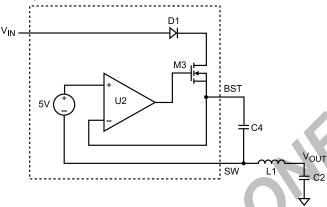
Figure 2—Internal Bootstrap Charging Circuit
