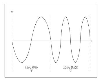
Figure 1. HART FSK Signal
