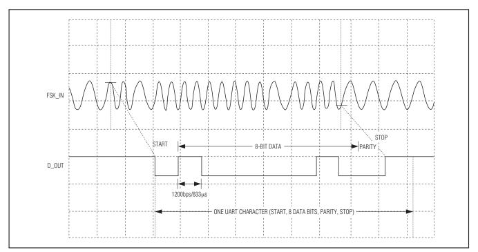
Figure 3. Actual DS8500 Demodulator Waveform
