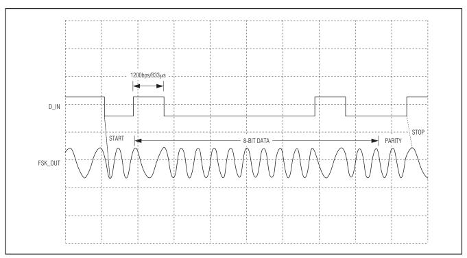
Figure 2. Actual DS8500 Modulator Waveform
