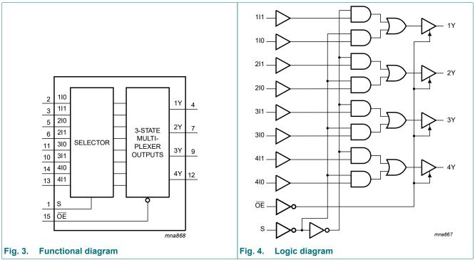
Quad 2-input multiplexer with 5 V tolerant inputs/outputs; 3-state
