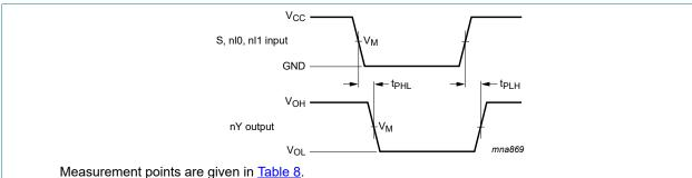
V<sub>OL</sub> and V<sub>OH</sub> are typical output voltage levels that occur with the output load.
