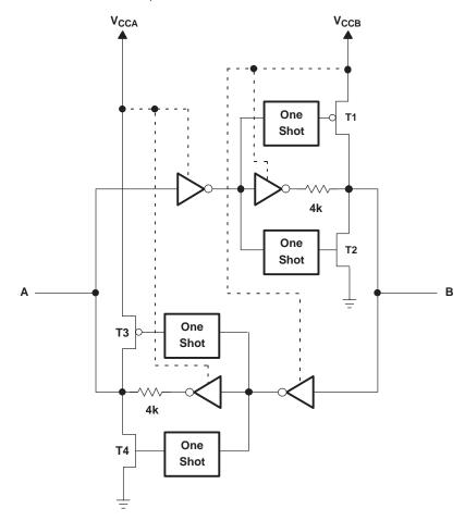
Figure 5. Architecture of TXB0102 I/O Cell
