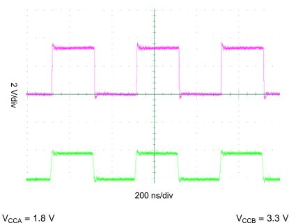
Figure 8. Level-Translation of a 2.5-MHz Signal
