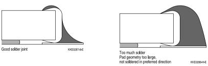
Good and poor solder joints caused by amount of solder in dual-wave soldering.
