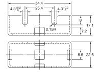
Note: The Cover has five holes for easy lead wire connections.
