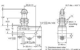
Note: Do not use the M12 mounting screw and the case mounting hole at the same time, or the case may be damaged.
