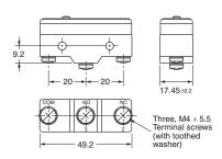
Note: With reverse action models (Z-15GM), the positions of NO and NC terminals are
