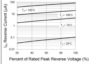
Fig.3 Typical Reverse Characteristics
