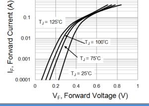
Fig.4 Typical Forward Characteristics
