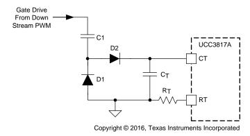
Figure 11. Synchronizing the UCC3817A to a Down-Stream Converter
