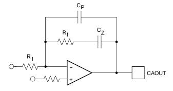
Figure 7. Current Loop Compensation
