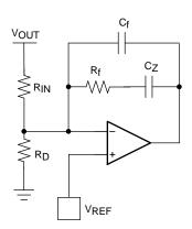
Figure 6. Voltage Amplifier Configuration
