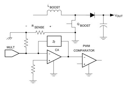
Figure 8. UCC3817A Current Amplifier Configuration
