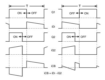
Figure 10. Timing Waveforms for Synchronization Scheme
