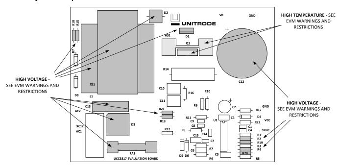
Figure 17. UCC3817EVM Evaluation Board Layout Assembly
