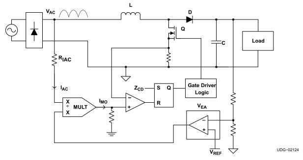
Figure 3. Basic Block Diagram of CRM Boost PFC
