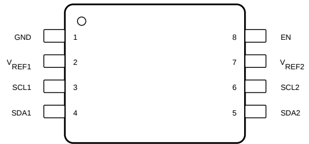
Figure 5-2. DCU Package 8-Pin VSSOP Top View
