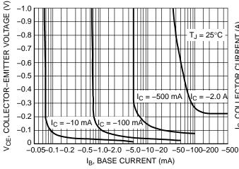
Figure 3. Collector Saturation Region
