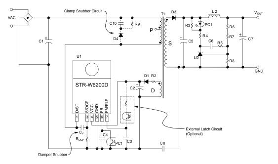
The following design feature should be observed: In applications having a power supply specified such that  $V_{DS}$  has large transient surge voltages, a clamp snubber circuit of a capacitor-resistor-diode (CRD) combination should be added on the primary winding, P, or a damper snubber circuit of a capacitor (C) or a resistor-capacitor (CR) combination should be added between the D/ST pins and the S/OCP pin.
