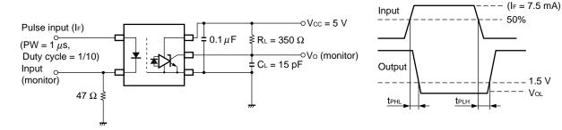
Remark C<sub>L</sub> includes probe and stray wiring capacitance.
