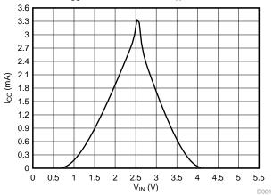
Figure 1.  $V_{\text{IN}}$  vs  $I_{\text{CC}}$
