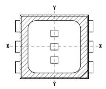
**Figure 14 Recommended Soldering Land Pattern**
