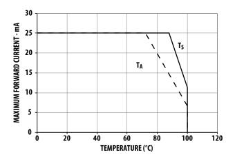
**NOTE** Maximum forward current graphs based on ambient temperature,  $T_A$  are with reference to thermal resistance  $R_{\theta J-A}$  as follows. For more details, see Precautionary Notes (4).
