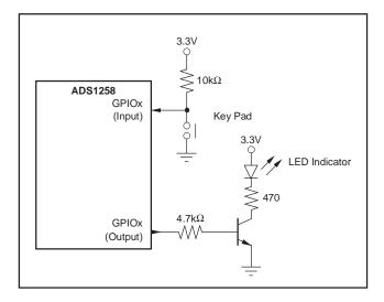
Figure 66. GPIO Connections
