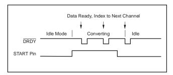
Figure 53. Conversion Control, Auto-Scan Mode
