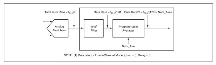
Figure 41. Block Diagram of Digital Filter
