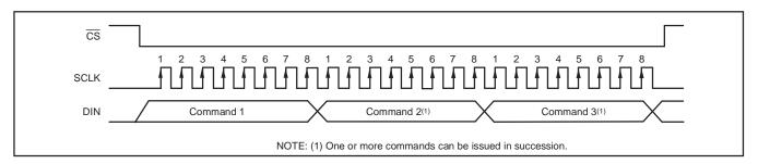
Figure 60. Control Command Operation
