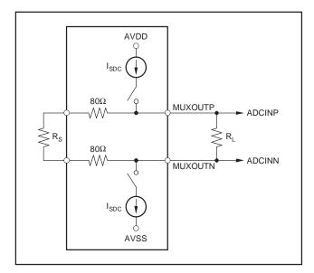
Figure 47. Sensor Bias Structure
