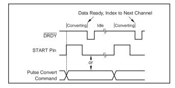
Figure 54. Pulse Conversion, Auto-Scan Mode
