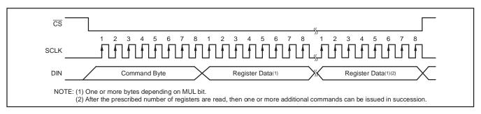
Figure 59. Register Write Operation
