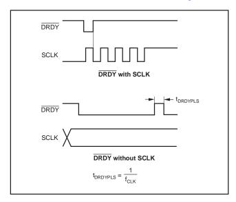
Figure 52. DRDY Timing (See Figure 2 for the DRDY Pulse)
