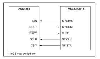
Figure 65. Connection to a TMS320R2811 DSP
