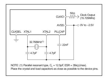
Figure 39. Crystal Oscillator Connection
