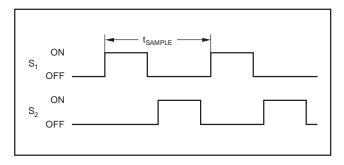
Figure 36. S<sub>1</sub> and S<sub>2</sub> Switch Timing for Figure 37
