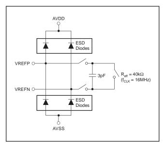
Figure 34. Simplified Reference Input Circuit
