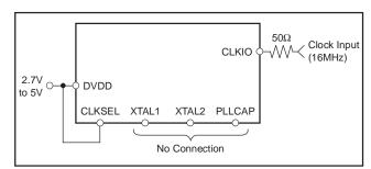
Figure 40. External Clock Connection
