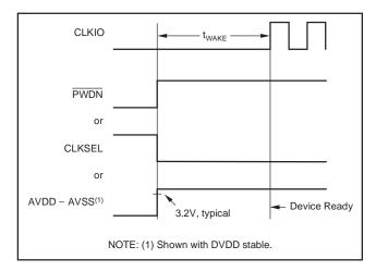
Figure 50. Device Wake Time with Internal Oscillator
