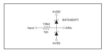
Figure 62. Input Overload Protection
