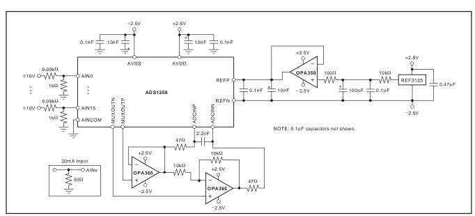
Figure 67. Multichannel, ±10V Single-Ended Input, Bipolar Supply Operation
