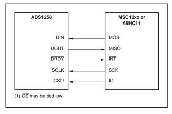
Figure 64. Connection to Microcontrollers with an SPI Interface
