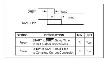
Figure 55. START Pin and DRDY Timing
