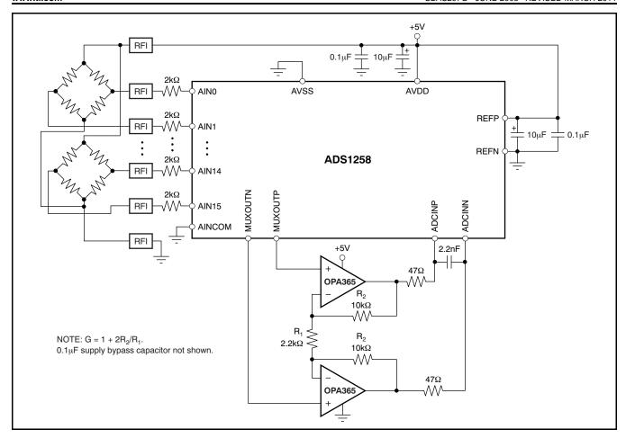
Figure 68. Bridge Input, Single-Supply Operation
