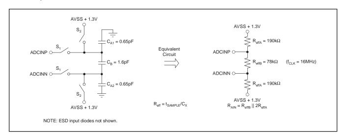
Figure 37. Simplified ADC Input Structure
