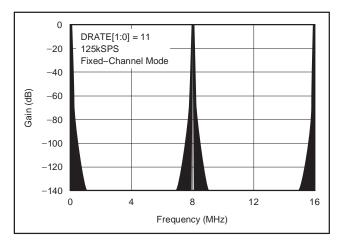
Figure 44. Frequency Response Out to 16MHz
