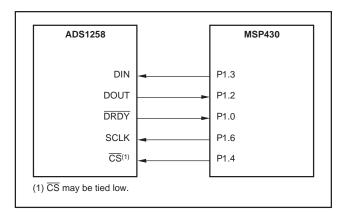
Figure 63. Connection to MSP430 Microcontroller
