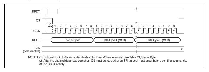
Figure 57. Channel Data Read Direct (No Command)
