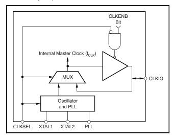
Figure 38. Clock Generation Block Diagram
